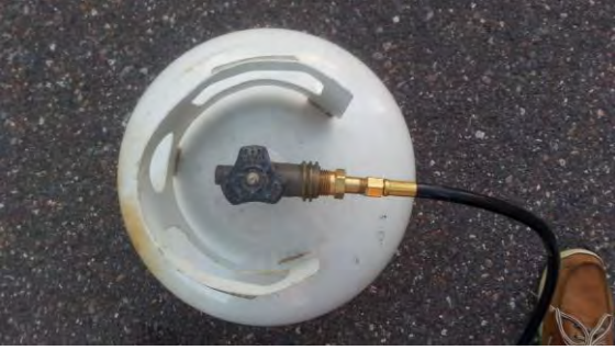
POL Valve on LP Tank
